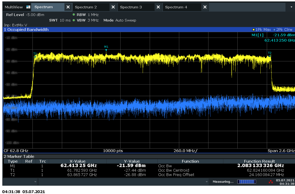
Spectrum Mask @ 50°C (2GHz profile)
