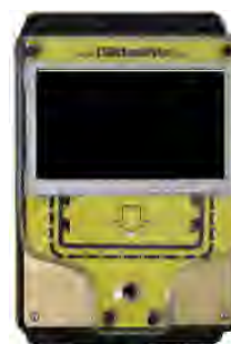
ESD Check Point Operator Panel
