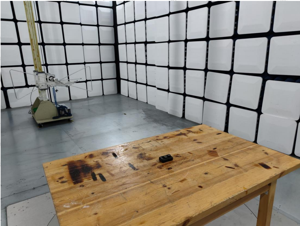
Photo of Radiation Emission Test
