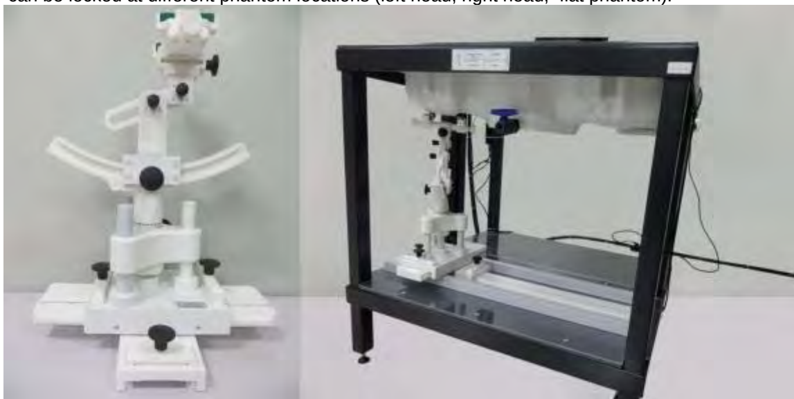
Device holder supplied by SATIMO
