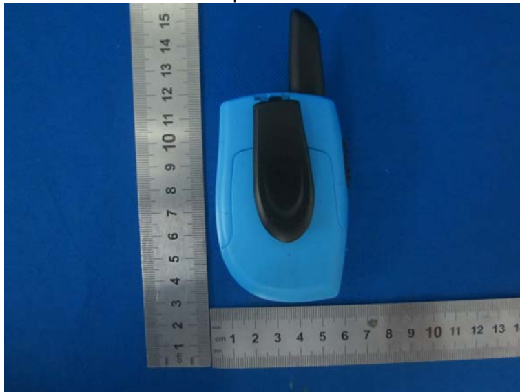
B1 – Battery, Intrinsically Safe Li-ion Battery
