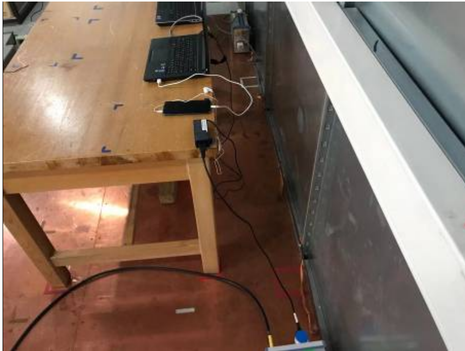
Conducted Emissions Test Setup (with laptop)
