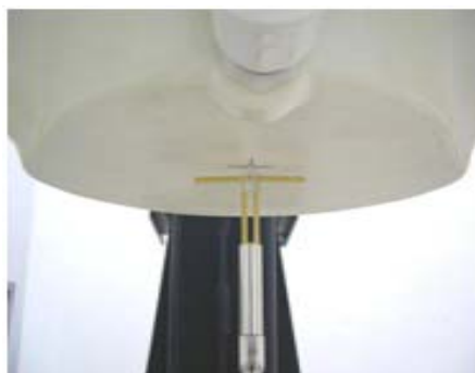
Fig 8.1 Photo of Dipole Setup Fig 8.2 System Setup for System Evaluation
