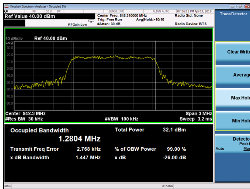
99% &amp; 26dB Occupied Bandwidth Plot on Channel 777
