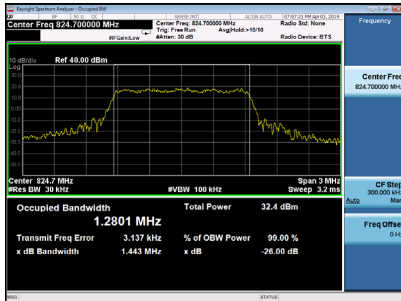
99% & 26dB Occupied Bandwidth Channel 1013
