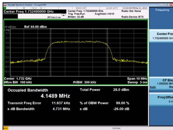
(Plot G2: WCDMA 1700MHz Channel = 1412 Occupied bandwidth)
