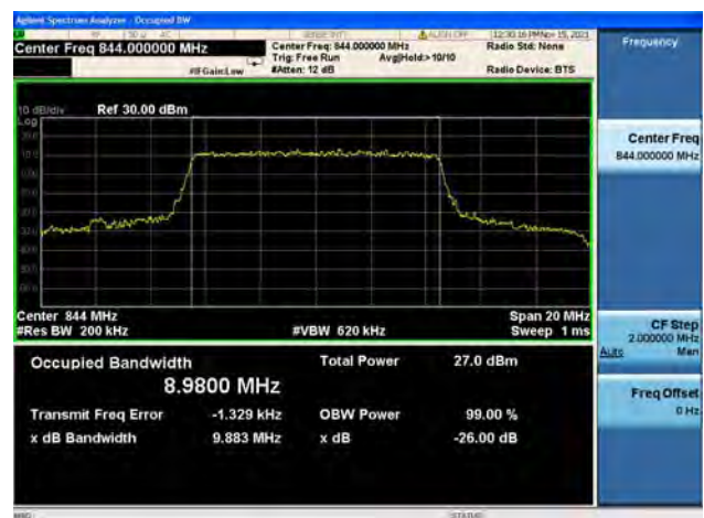
Band26 / 10MHz / High CH / 64QAM
