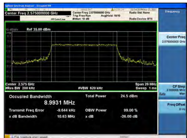
Band38 / 10MHz / Low CH / 64QAM
