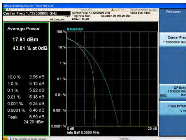
Band4 / 5MHz / Mid CH / 16QAM
