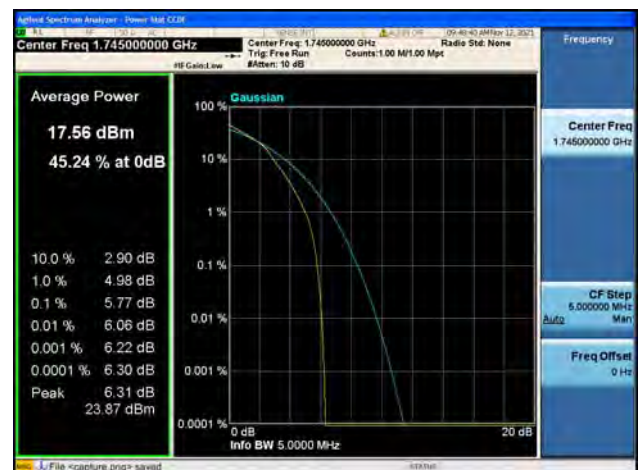
Band66 / 5MHz / Mid CH / 64QAM
