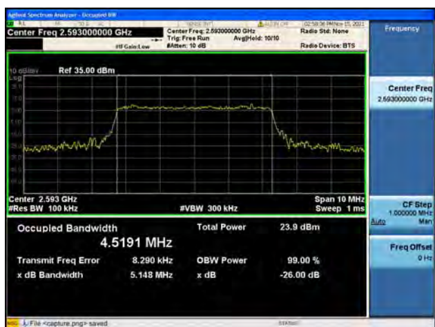
Band41 / 5MHz / Mid CH / 16QAM
