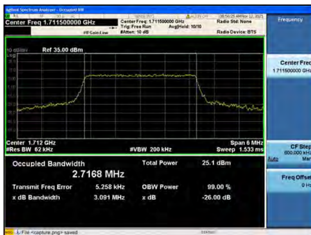
Band66 / 3MHz / Low CH / 16QAM
