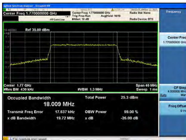
Band66 / 20MHz / High CH / 16QAM
