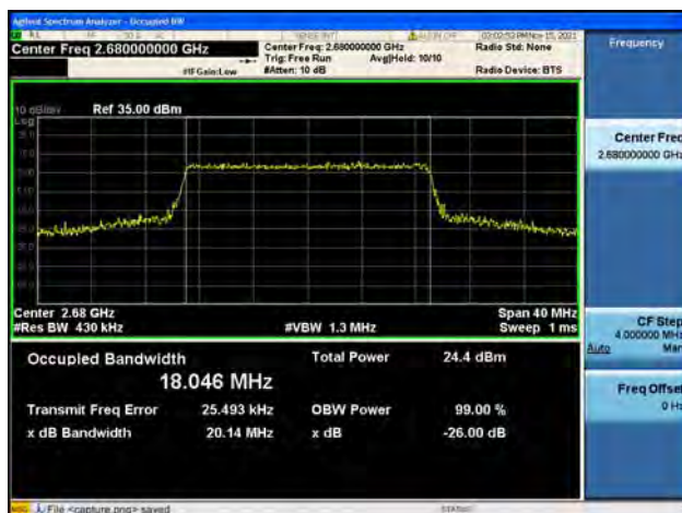
Band41 / 20MHz / High CH / 16QAM
