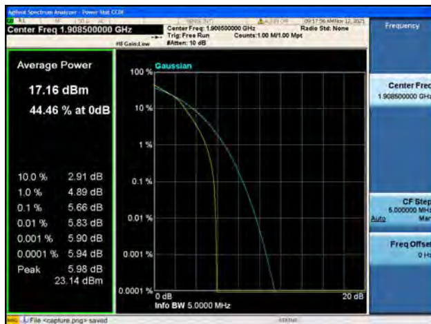
Band2 / 3MHz / High CH / 16QAM
