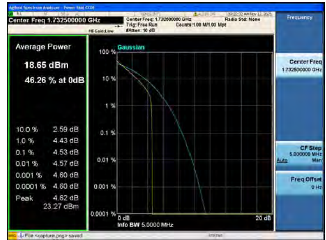
Band4 / 1.4MHz / Mid CH / 64QAM
