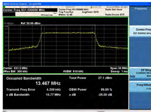
Band26 / 15MHz / Low CH / 64QAM
