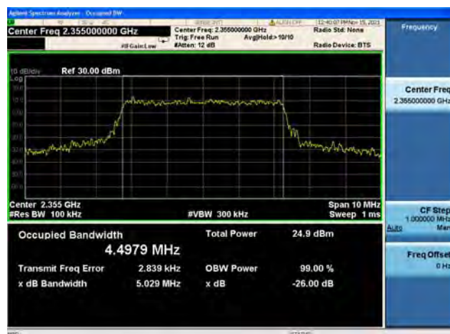
Band40/ Block B / 5MHz / Mid CH / 16QAM
