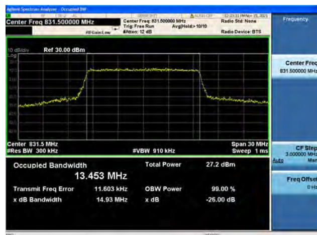
Band26 / 15MHz / Mid CH / 16QAM
