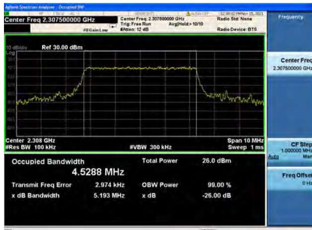
Band40/ Block A / 5MHz / Mid CH / 16QAM
