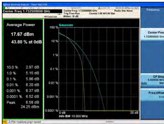
Band4 / 10MHz / High CH / 16QAM
