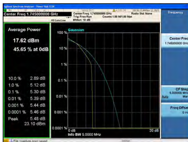
Band66 / 1.4MHz / Mid CH / 16QAM
