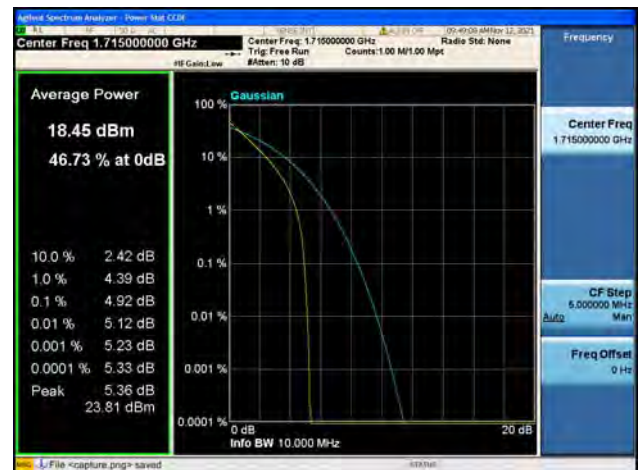
Band66 / 10MHz / Low CH / 64QAM
