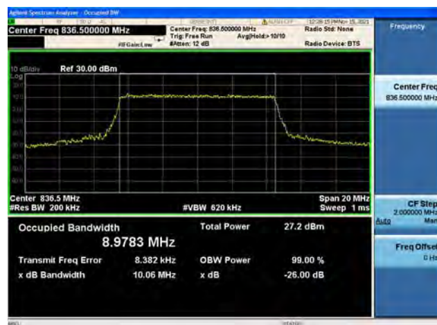
Band26 / 10MHz / High CH / 16QAM
