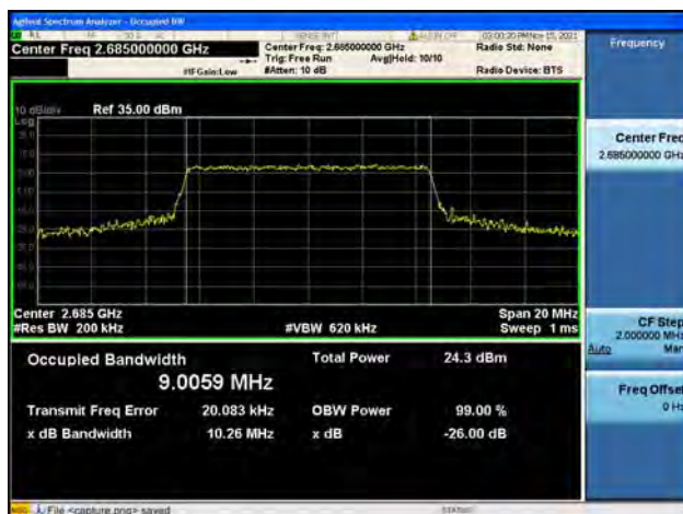
Band41 / 10MHz / High CH / 16QAM
