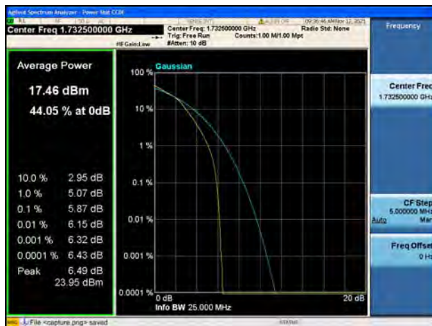
Band4 / 20MHz / High CH / 16QAM
