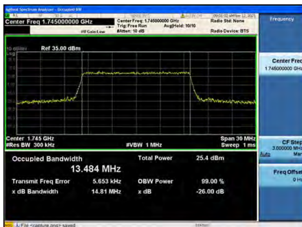
Band66 / 15MHz / Mid CH / 16QAM
