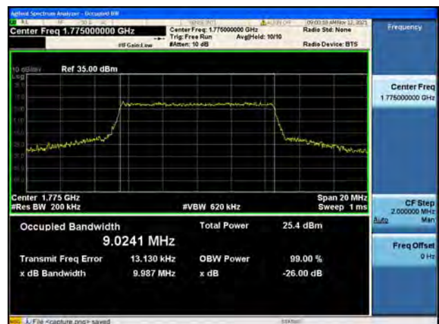
Band66 / 10MHz / High CH / 64QAM
