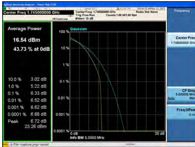
Band66 / 3MHz / High CH / 16QAM
