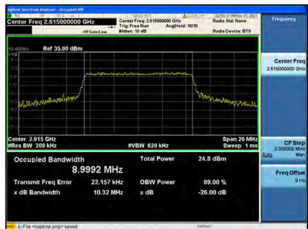
Band38 / 10MHz / High CH / 64QAM
