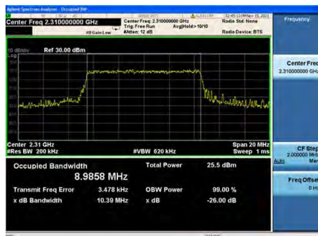
Band40/ Block A / 10MHz / Mid CH / 16QAM
