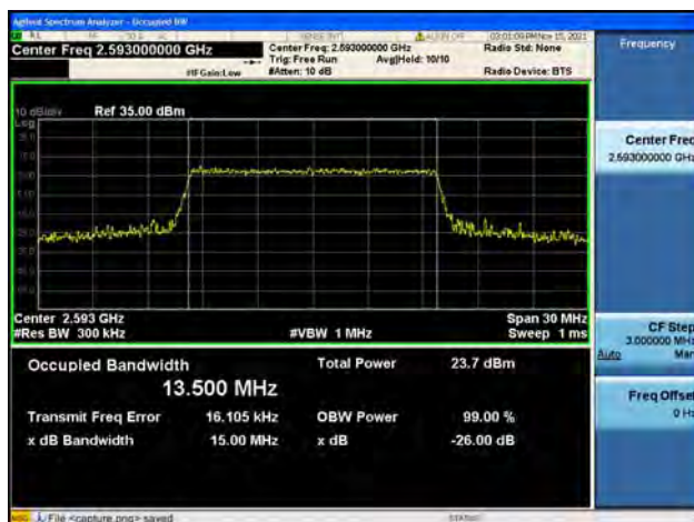
Band41 / 15MHz / Mid CH / 16QAM
