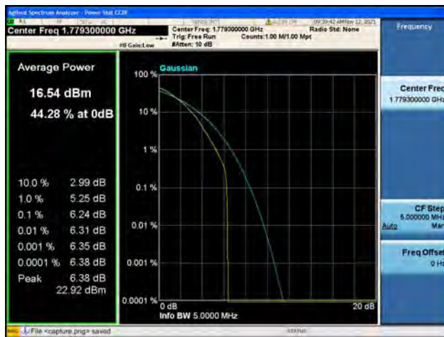
Band66 / 3MHz / Low CH / 16QAM
