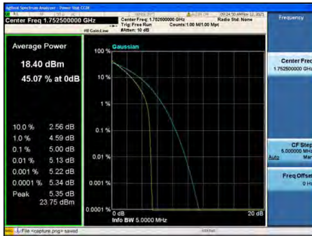
Band4 / 5MHz / High CH / 64QAM
