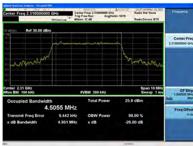
Band40/ Block A / 5MHz / Mid CH / 16QAM
