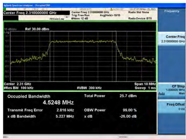
Band40/ Block A / 5MHz / Mid CH / 64QAM
