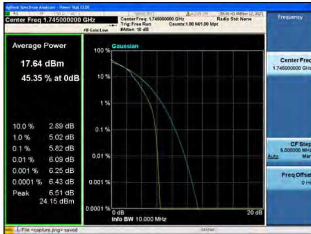
Band66 / 10MHz / High CH / 16QAM
