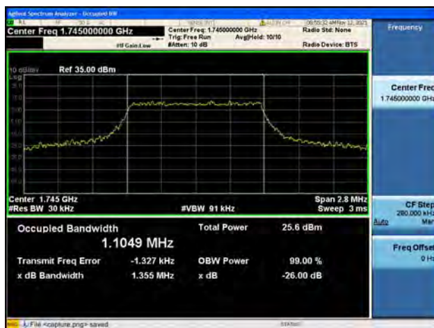
Band66 / 1.4MHz / Mid CH / 16QAM
