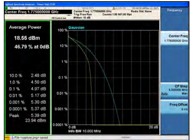
Band66 / 10MHz / High CH / 64QAM
