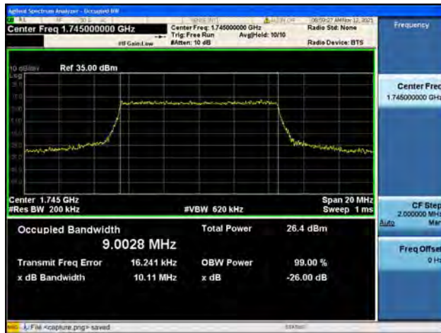
Band66 / 10MHz / Mid CH / 64QAM
