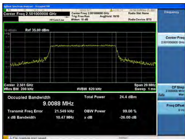
Band41 / 10MHz / Low CH / 64QAM
