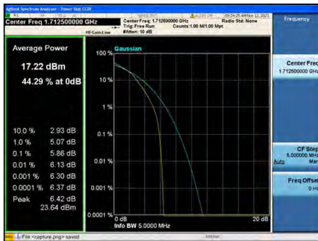
Band4 / 5MHz / Mid CH / 16QAM
