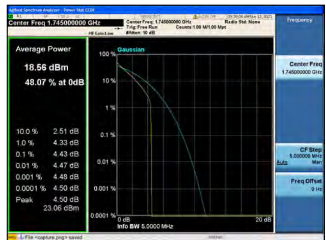
Band66 / 1.4MHz / Mid CH / 64QAM
