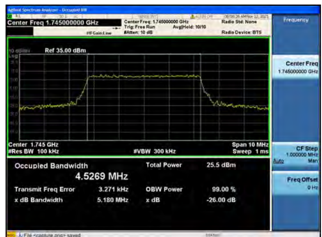
Band66 / 5MHz / Mid CH / 64QAM
