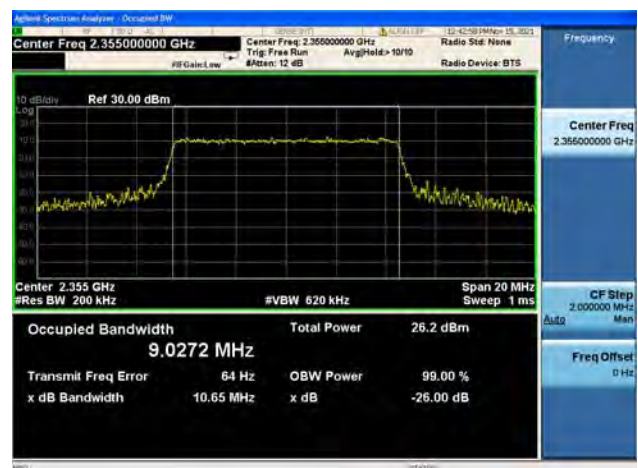
Band40/ Block B / 10MHz / Mid CH / 64QAM
