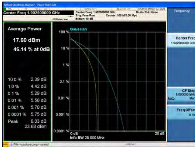
Band2 / 15MHz / High CH / 64QAM
