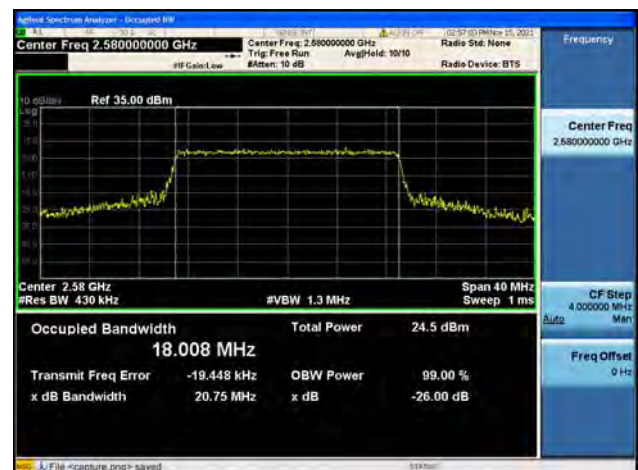
Band38 / 20MHz / Low CH / 64QAM
