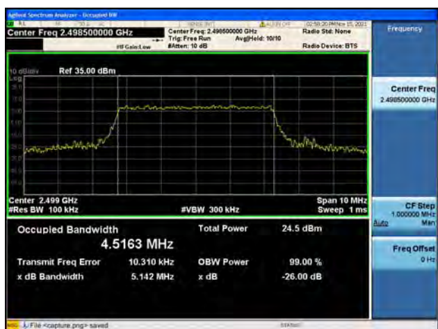
Band41 / 5MHz / Mid CH / 16QAM
