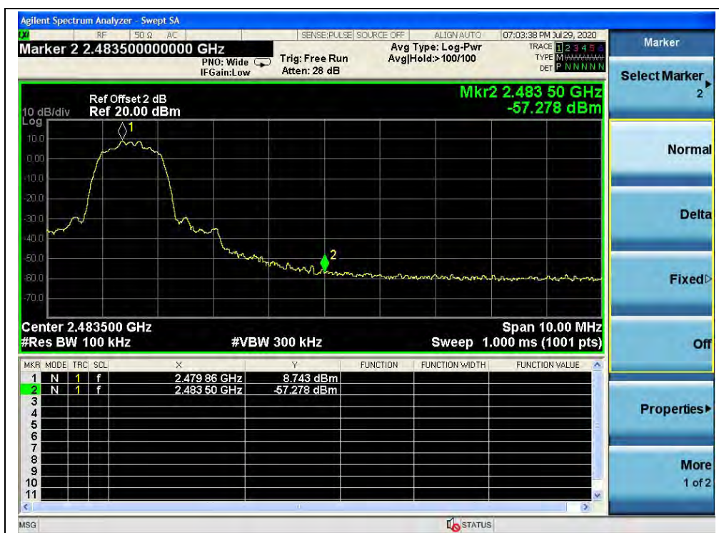
(Band edge, Channel 78, \pi/4 -DQPSK)
