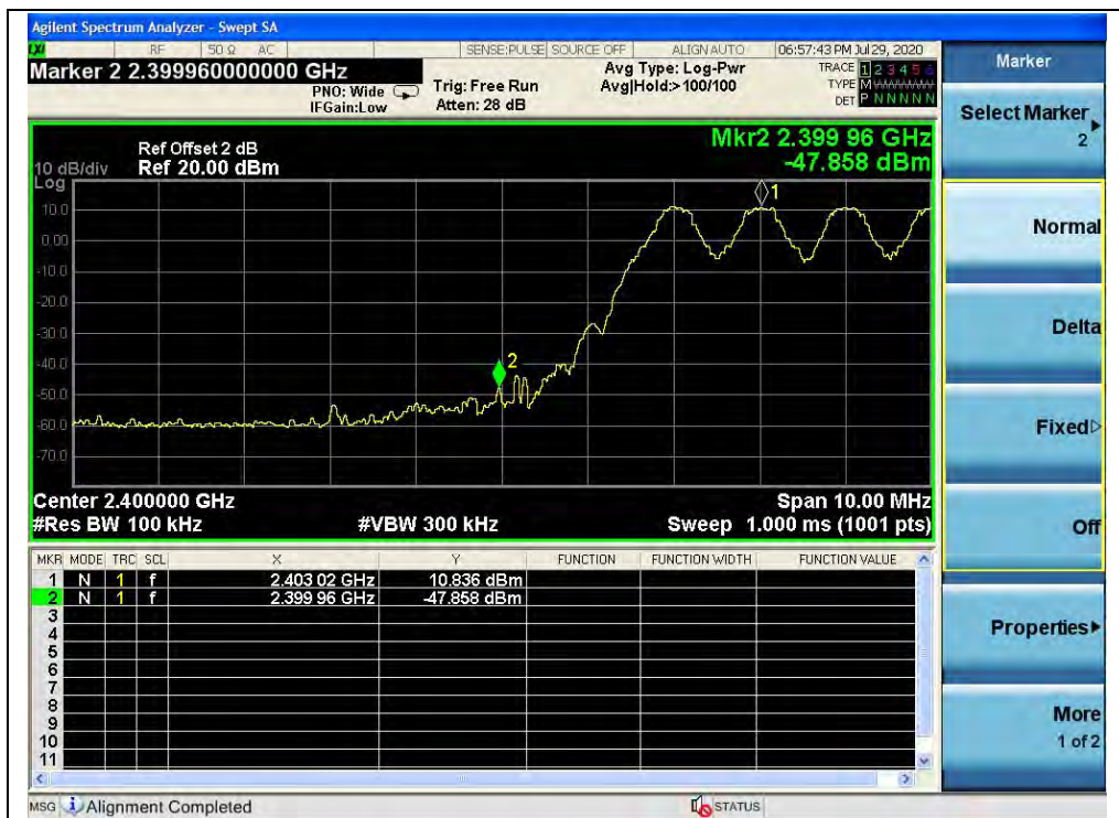
(Band edge with hopping on, Channel 0, GFSK)
