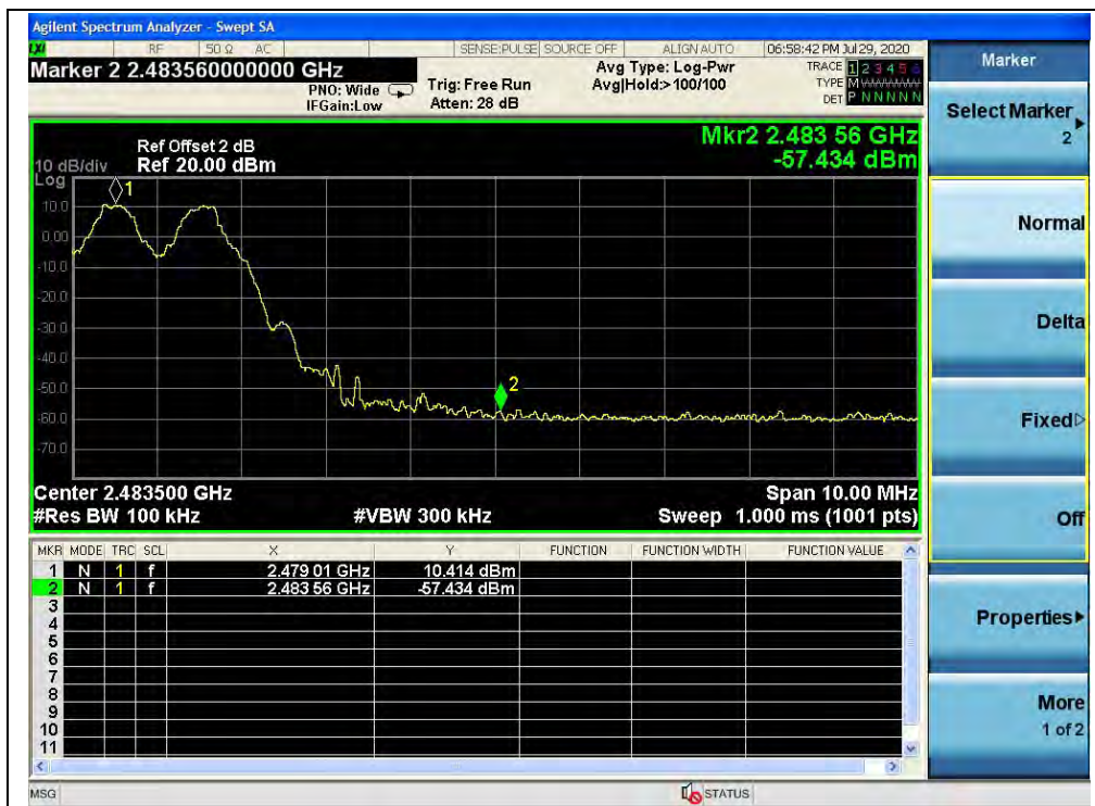
(Band edge with hopping on, Channel 78, GFSK)
