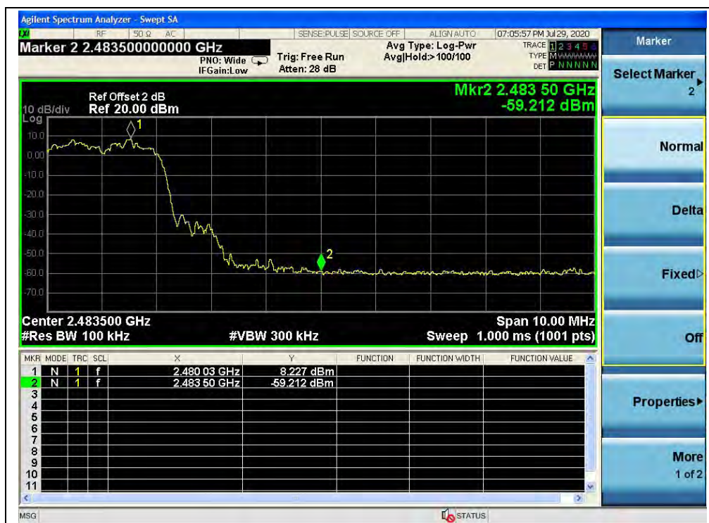
(Band edge with hopping on, Channel 78, 8-DPSK)
