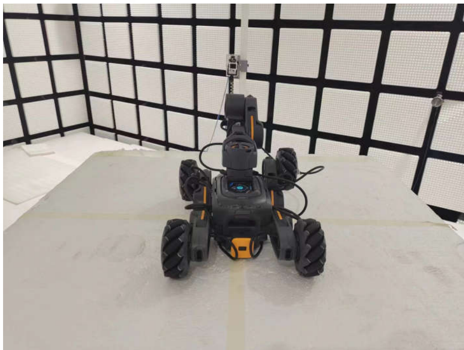
Radiated spurious emission Test Setup-3(Above 18GHz)
