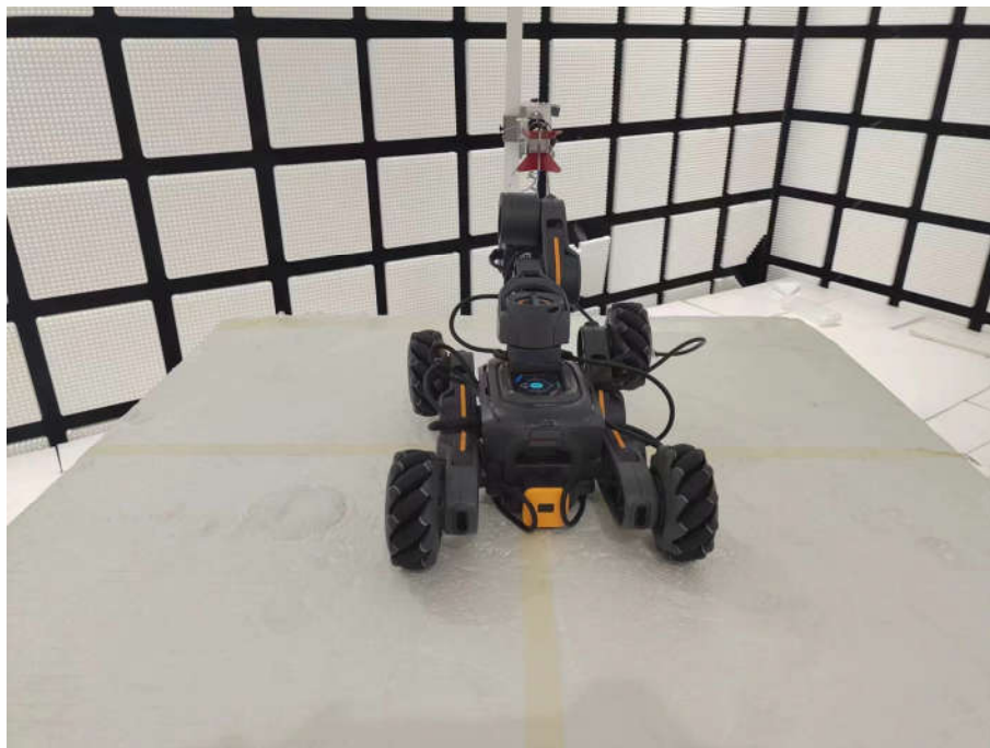
Radiated spurious emission Test Setup-2(Above 1GHz)
