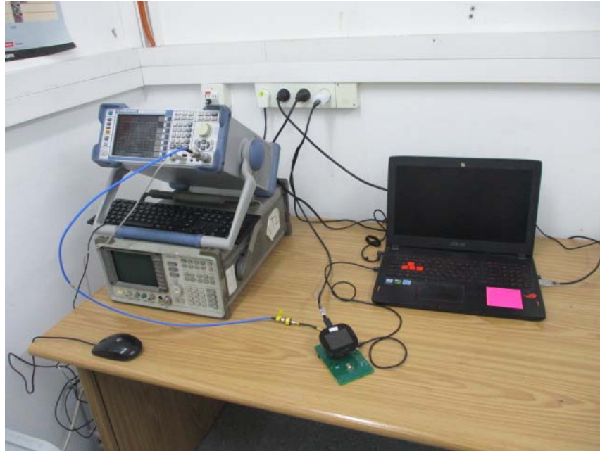
Figure 4. Conducted Test Set Up
