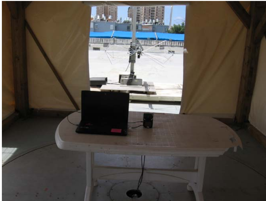
Figure 6. Radiated Emission Test, 30-200MHz
