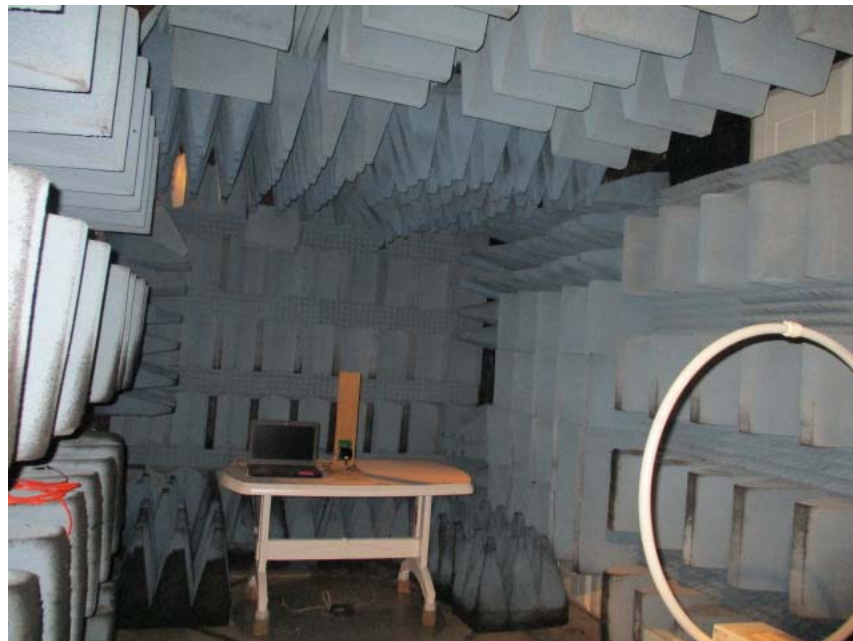
Figure 5. Radiated Emission Test, 0.009-30MHz
