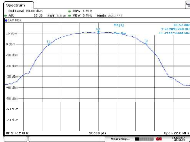
802.11b 99% Occupied Bandwidth (Channel 1)
