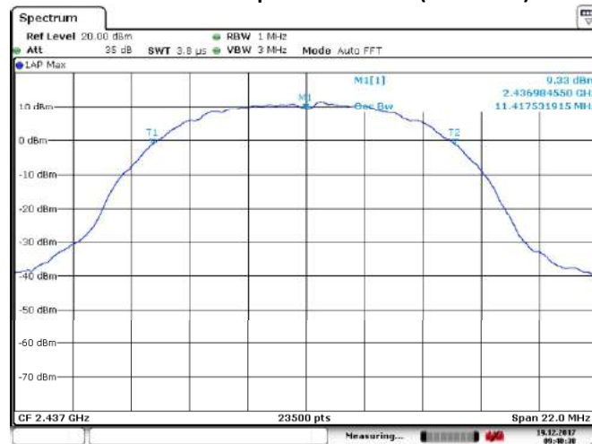
802.11b 99% Occupied Bandwidth (Channel 6)
