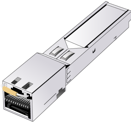
Figure 4-2 Copper SFP Module
