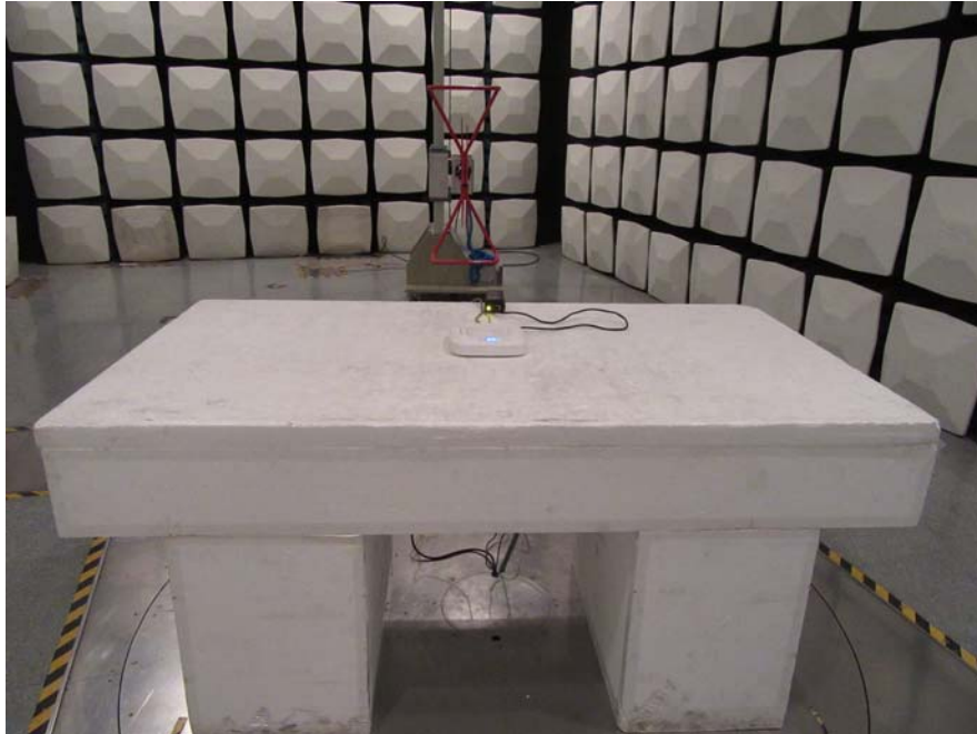
Radiated Emission View (Below 1 GHz)
