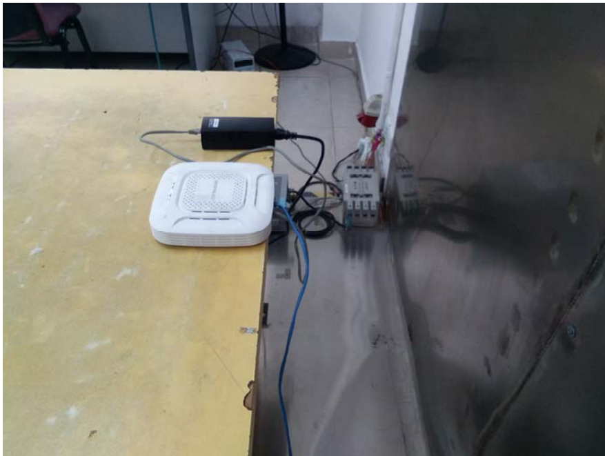
Conducted Emission Rear View
