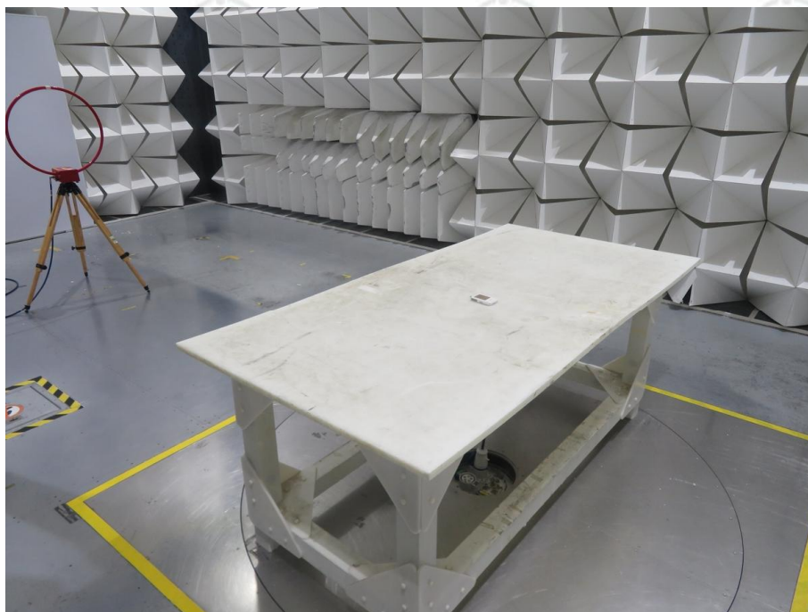
Radiated emission Test Setup-5(Below 30M)
