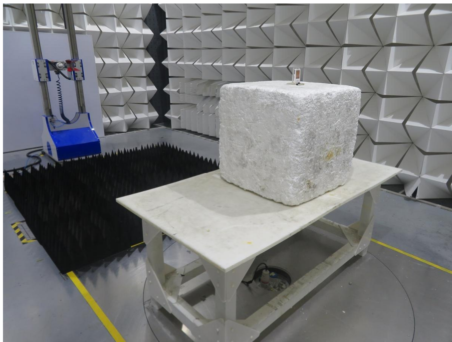
Radiated spurious emission Test Setup-2(Above 1GHz)
