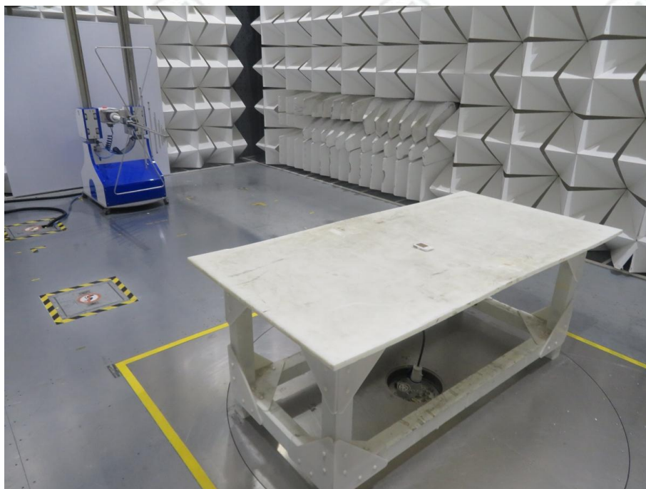
Radiated emission Test Setup-3(Below 1GHz)
