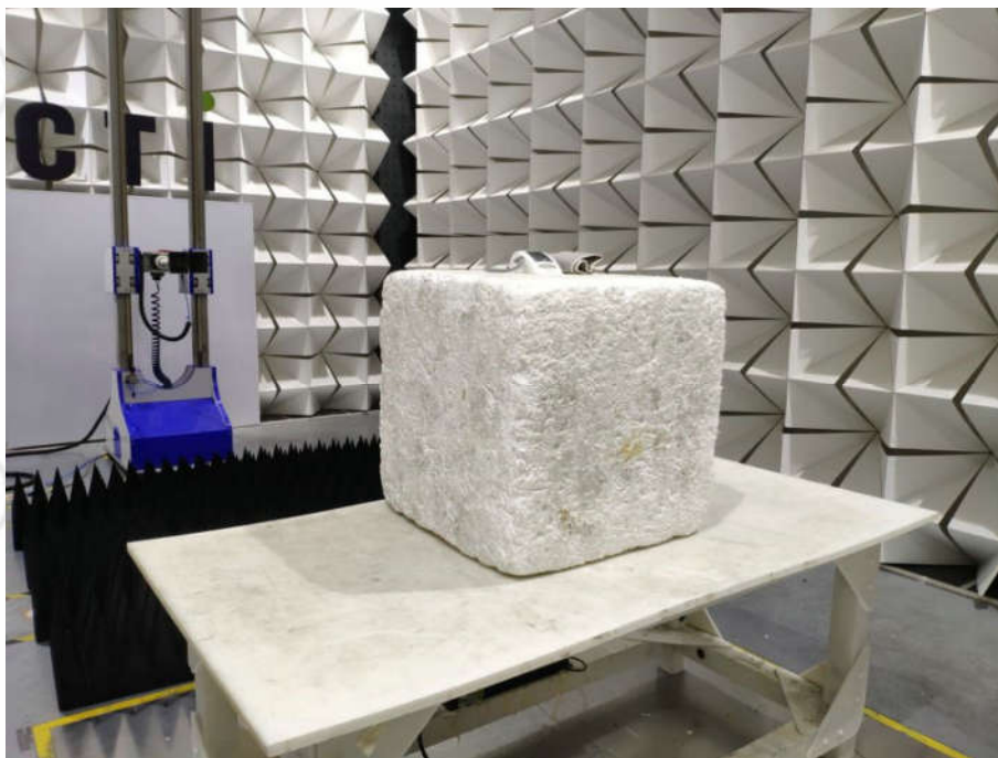
Radiated spurious emission Test Setup-2(Above 1GHz)
