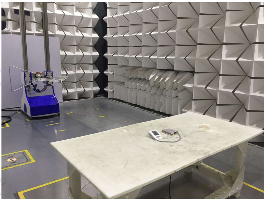
Radiated spurious emission Test Setup-1(Below 1GHz)
