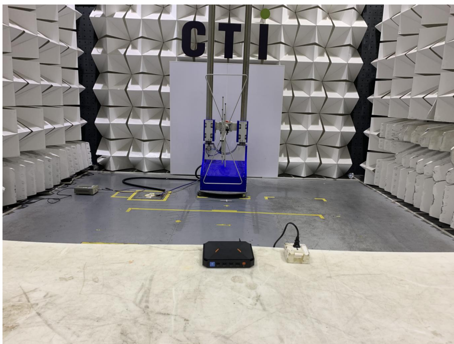
Radiated spurious emission Test Setup-2(Below 1GHz)
