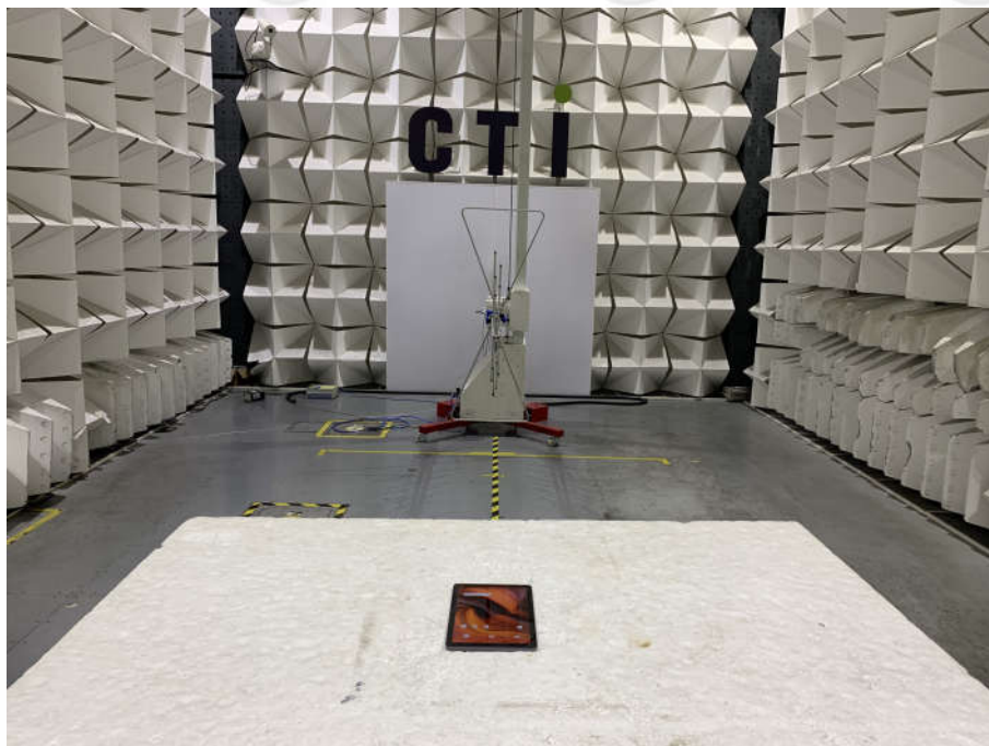
Radiated spurious emission Test Setup-1(Below 1GHz)
