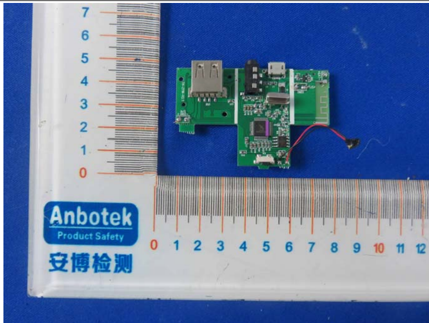
PCB of the EUT-Front View
