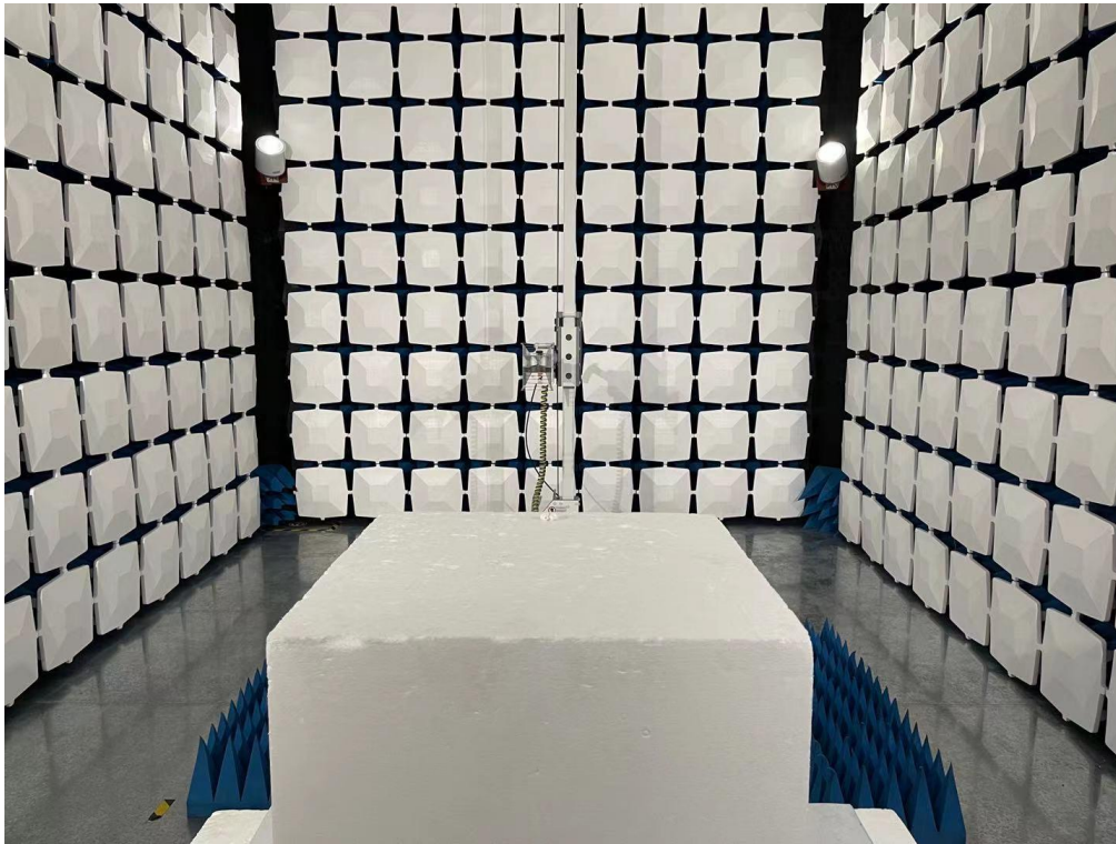
Above 1GHz for radiated emission test setup
