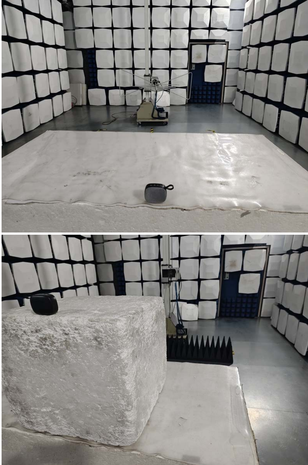
Radiated emission test view
