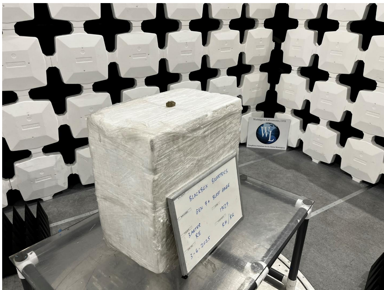
Radiated Testing, 1GHz to 12GHz, View 2
