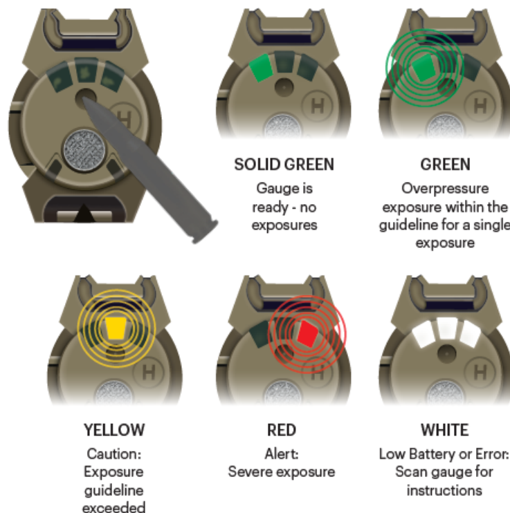
Figure 4: Manual Reading (LED Indicator)
