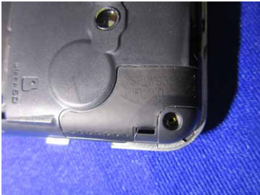
EUT- Wifi & BT Antenna View
