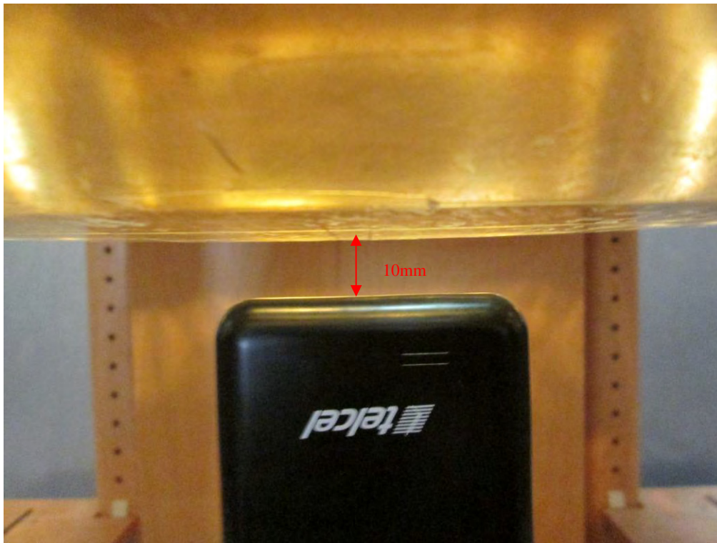
Body-worn Bottom Setup Photo (10mm)
