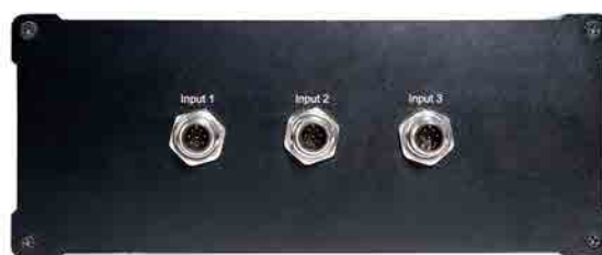
Figure 151 - The rear panel of LPIT test box
