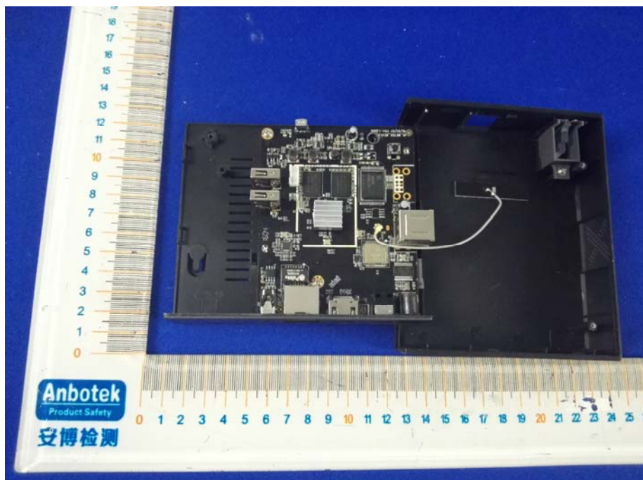
Figure 8 The EUT-Inside View
