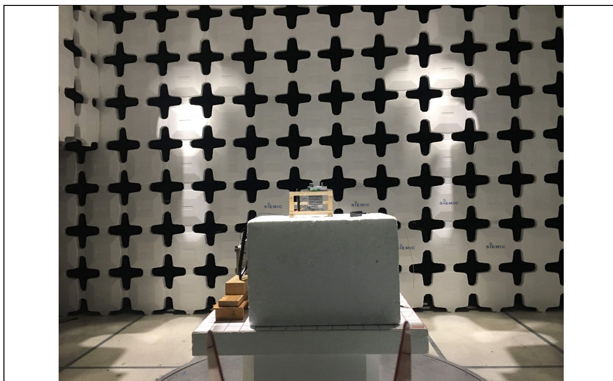
Radiated Emission Test above 1GHz Front View
