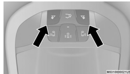
Courtesy Light Switches
