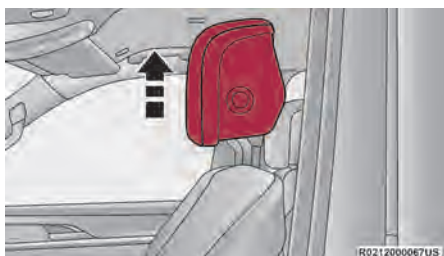
Upward Adjustment (Manual Head Restraint)
