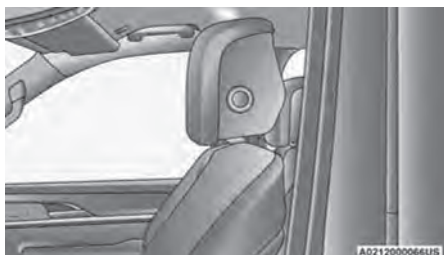
Upright Position (Manual Head Restraint)
