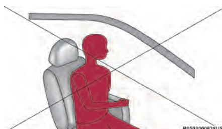
Not Seated Properly
