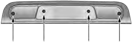
CHMSL Mounting Screw Locations
