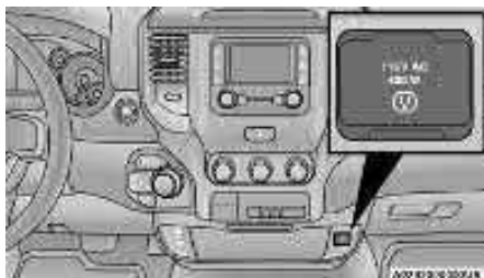
Center Stack Power Inverter
