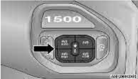
Five-Position/On-Demand Transfer Case — GT Models
