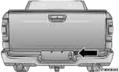
Access Hole Cover Location
