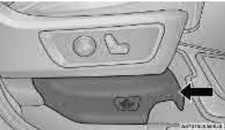
Pull Jack Access Cover From Front
