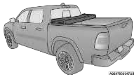
Position One (Front Latches Latched And Stowage Straps Secured)
