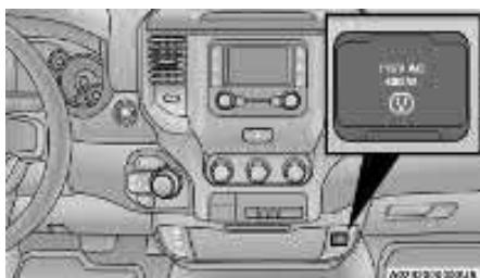
Center Stack Power Inverter
