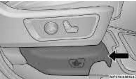
Pull Jack Access Cover From Front
