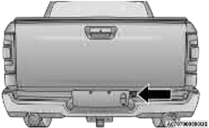
Access Hole Cover Location
