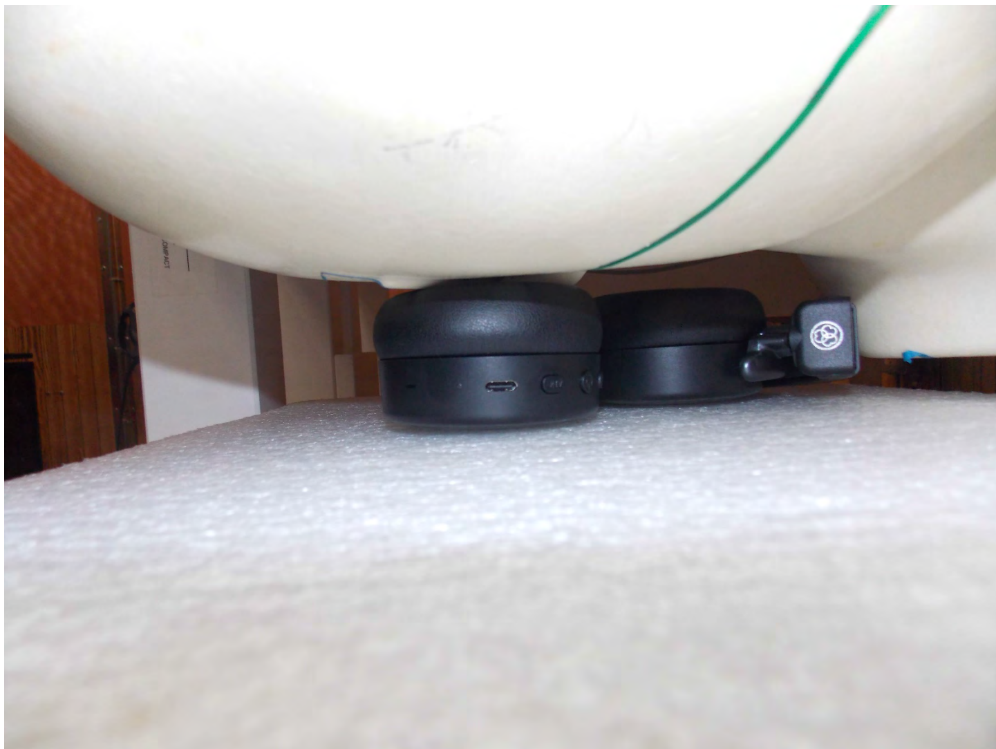
Test Position Next to Ear 0 mm Gap
