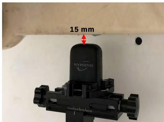
Fig.5 EUT Top side to flat phantom
