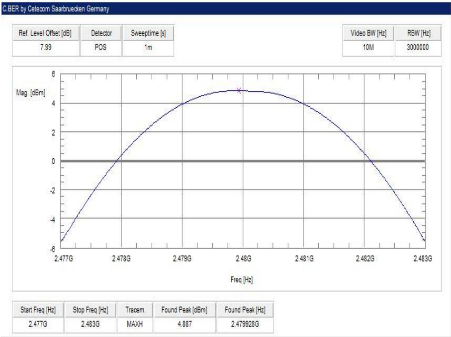
Plot 3: highest channel – 2480 MHz, GFSK modulation
