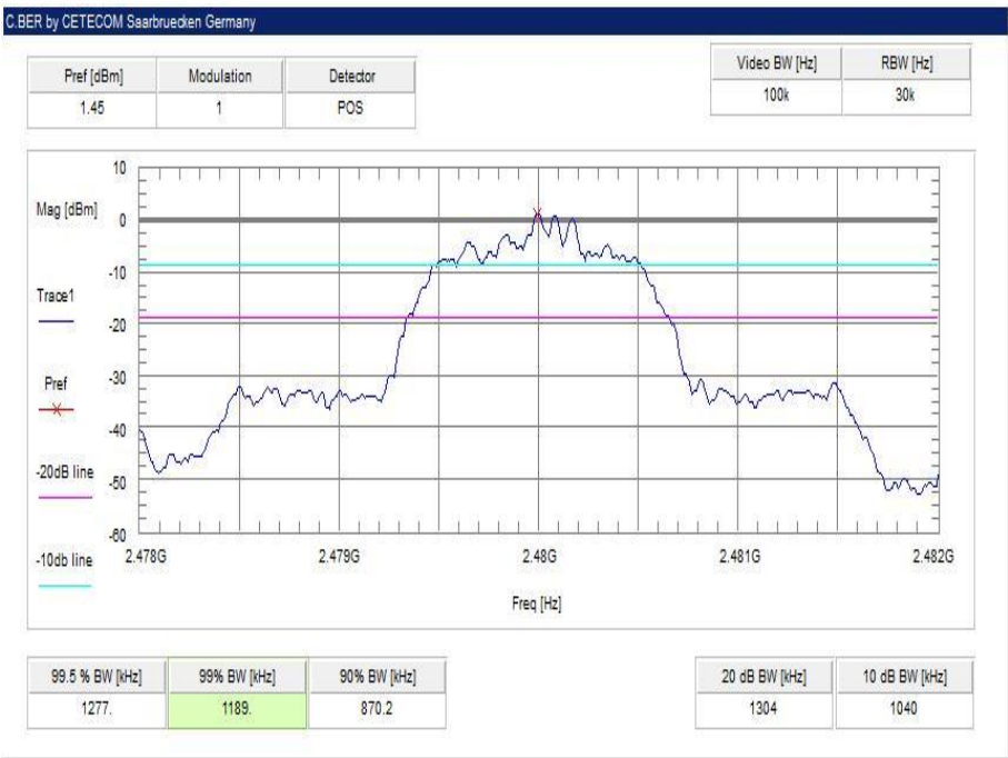
Plot 6: highest channel – 2480 MHz, Pi / DQPSK modulation
