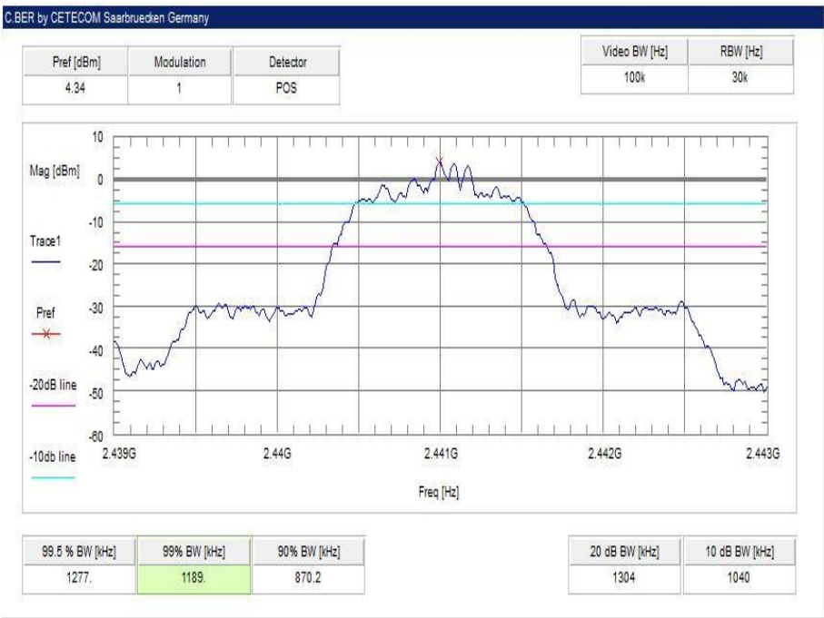
Plot 5: middle channel – 2441 MHz, Pi / DQPSK modulation
