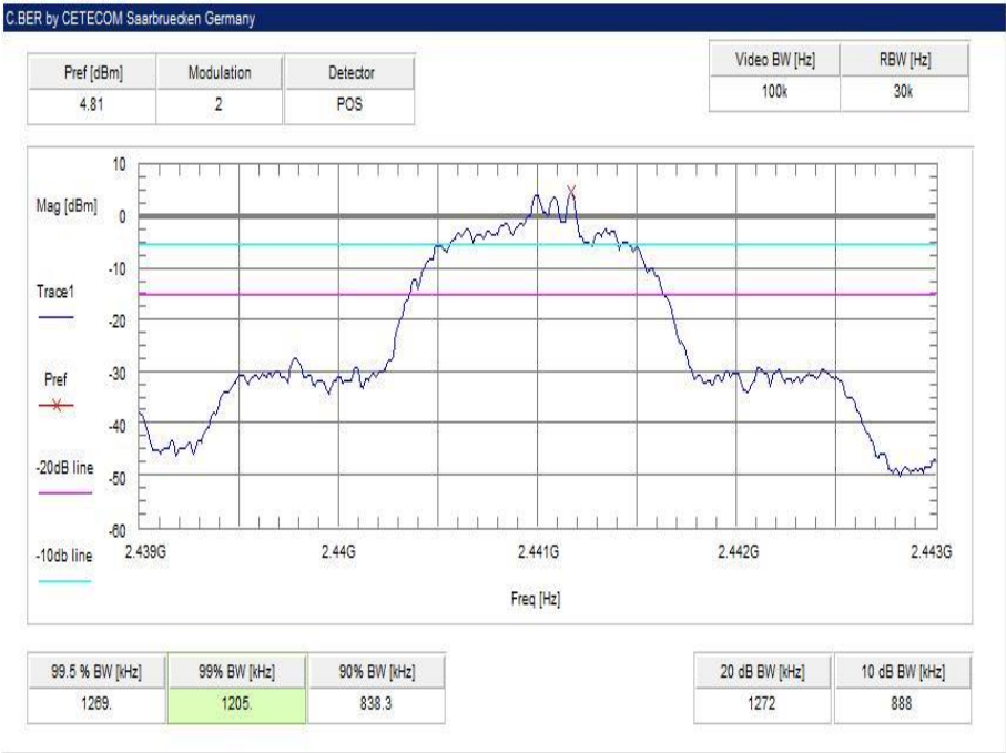
Plot 8: middle channel – 2441 MHz, 8 DPSK modulation
