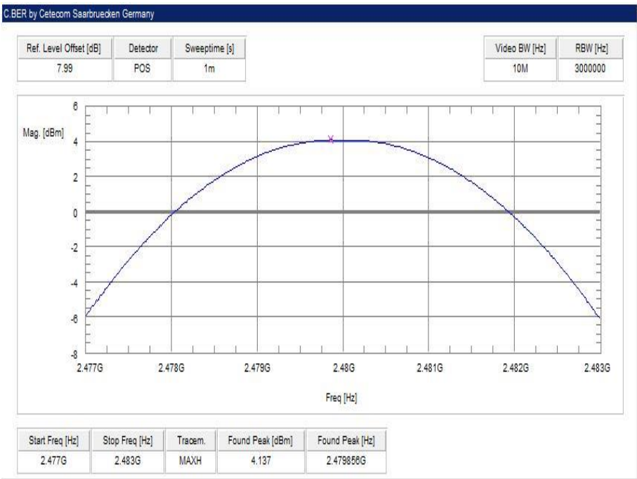
Plot 6: highest channel – 2480 MHz, Pi / DQPSK modulation
