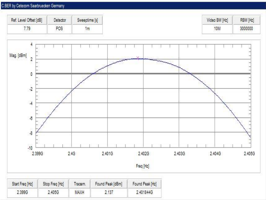
Plot 4: lowest channel – 2402 MHz, Pi / DQPSK modulation
