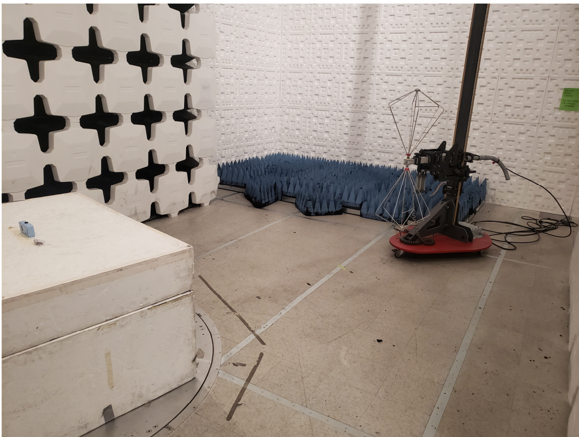
Figure 3. Radiated Emissions Test Setup, Intentional, 30 MHz to 200 MHz
