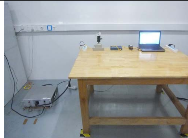
Conducted Emissions Test Setup Front View
