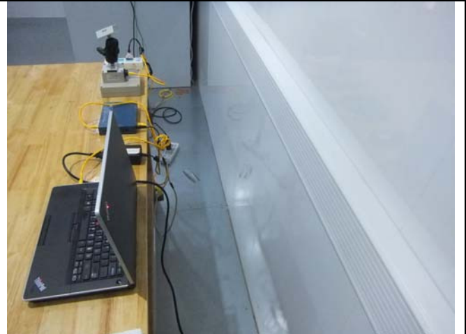
Conducted Emissions Test Setup Side View
