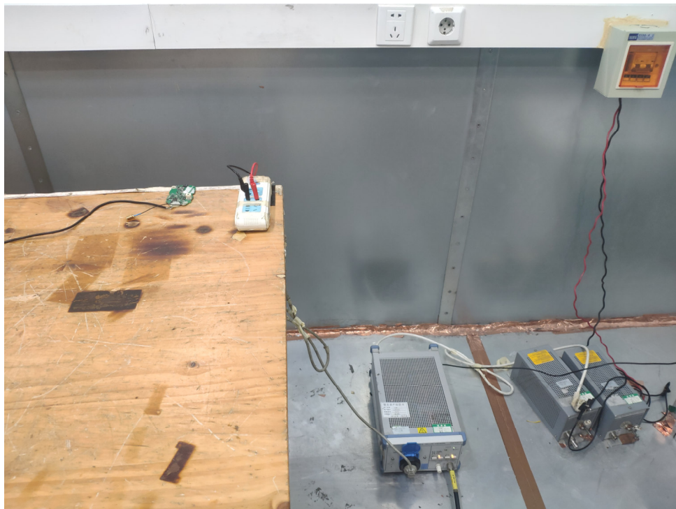
Picture 2 Conducted Emission Test Setup
