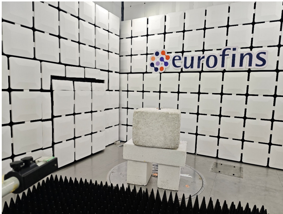
Picture 1 Radiated Emission Test Setup
