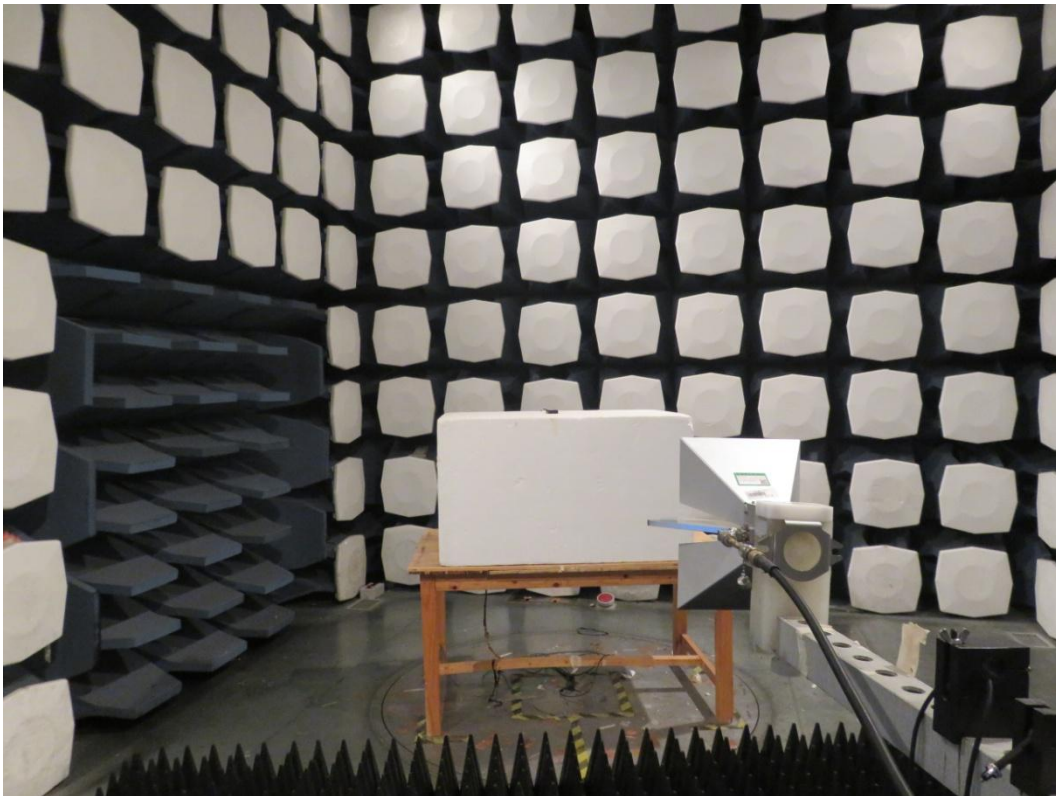
Picture 2: Radiated Spurious Emissions Test setup
