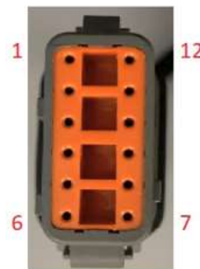
DTM06-12sa Harness native to FJ2500LA-12D and FJ2500MG-12D.
