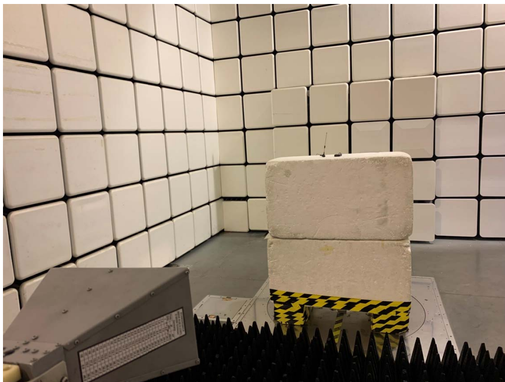
Picture 1: Radiated Spurious Emissions Test setup
