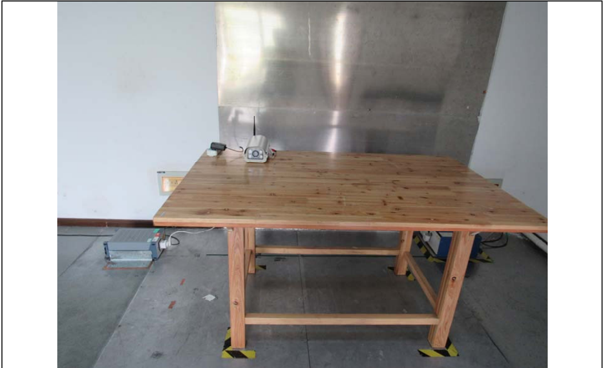
Conducted Emissions Setup Front View
