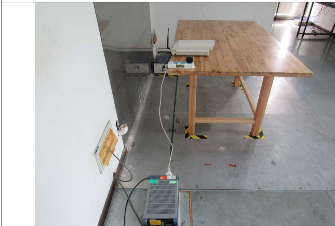
Conducted Emissions Setup Side View
