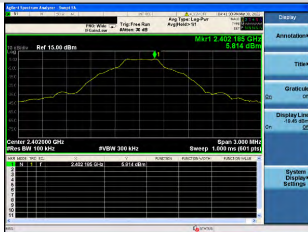
GFSK LOW CHANNEL, CARRIER LEVEL
