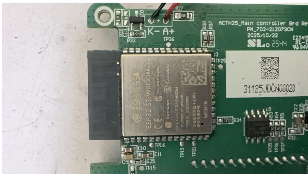
RF Module and Antenna
