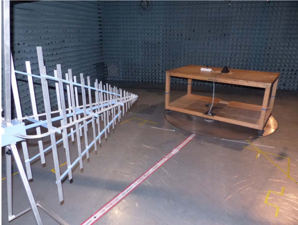
Photo 6: Test setup for radiated measurements (AC Port (power line), EUT supplied by AC/DC adapter, unintentional radiator §15.109, ANSI C63.4)
