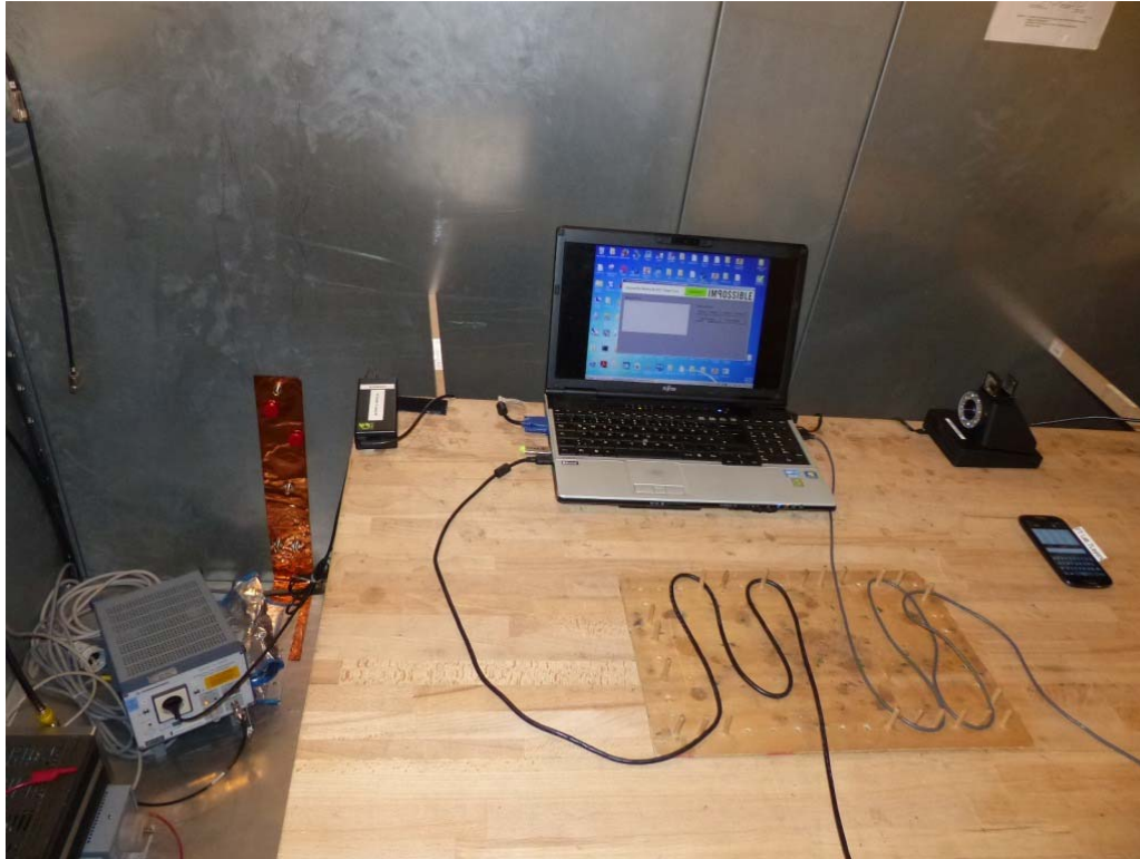
Photo 5: Test setup for conducted measurements (computer peripheral setup, EUT supplied by USB-cable from computer, unintentional radiator §15.107, ANSI C63.4)
